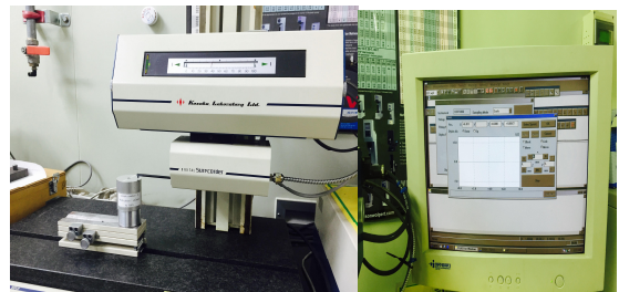
Fig. 7 Surface roughness measurement for shape meter(DSF-1000)
