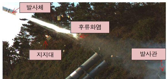
Fig. 5. Minimum & maximum thrust tests
