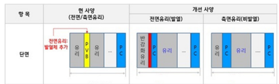
Fig. 7. The result of lamination layer's improvement
