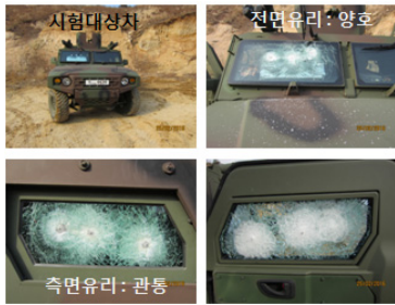
Fig. 6. The firing test result of KLTV glass(1 st )
