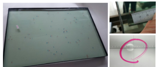
Fig. 4. The environmental test result of Iraq bullet-proof vehicle's glass
