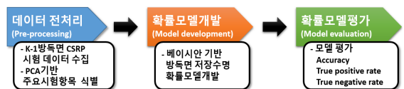
Fig. 3. Three stages for the shelf life estimation of the K-1 gas mask; pre-processing, and probability model development and model evaluation
