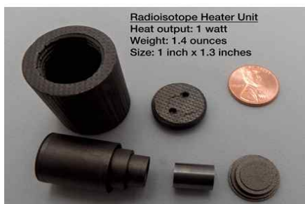
Fig. 3. Configuration of LWRHU[3]
