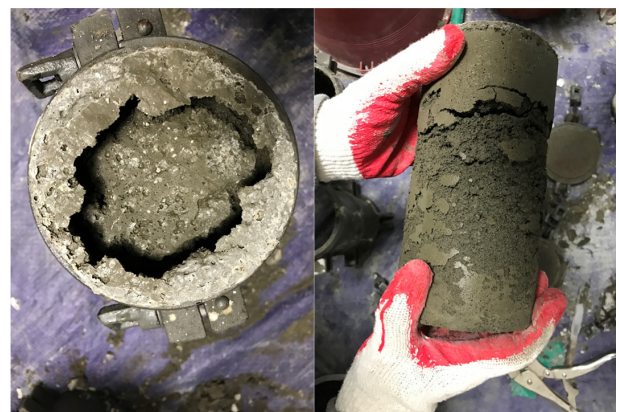
Fig. 7. Examples for non-homogeneous air distribution in specimens
