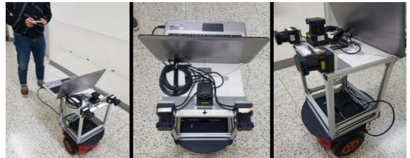
Fig. 1. Laser scanning system for acquiring 3D point cloud
