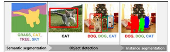
Fig. 9. Progress of CNN: From object detection to instance segmentation
