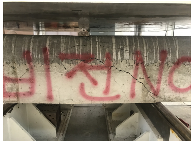
Photo 3. Cracks of non-composite additional wall during bending test (N-B-3)
