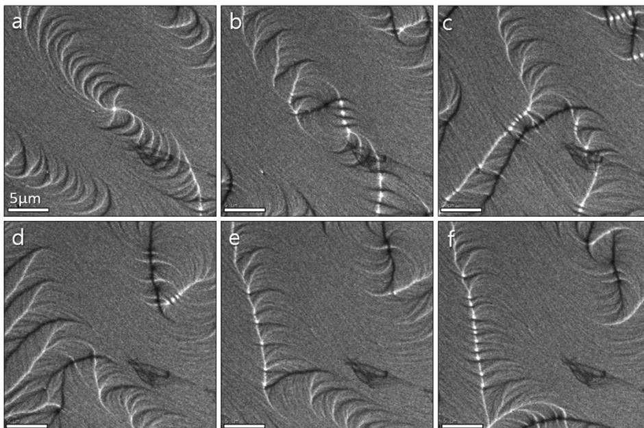
Domain wall motions (Chikazumi, 1997) were *in situ* observed by Lorentz microscopy (Caltech's second-generation ultrafast electron microscope: Zewail et al., 2010). Polycrystalline thin film layers of Ni on Ti (30 nm/30 nm) were deposited sequentially by electron beam evaporation onto a Si<sub>3</sub>N<sub>4</sub> membrane (15 nm thick, 0.25×0.25 mm<sup>2</sup> window). To trigger the domain wall motions,
