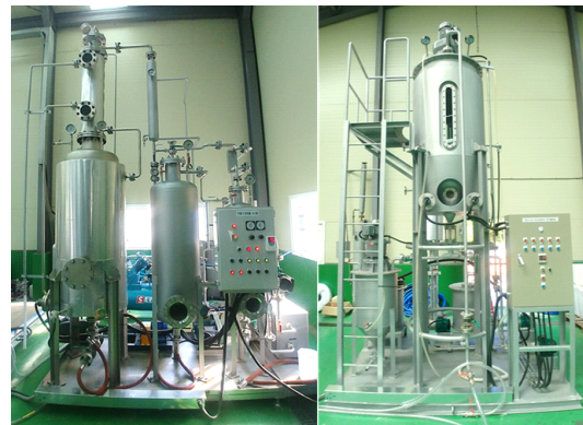
Fig. 2. Vacuum distillation apparatus (left) and deacidifying apparatus (right).
