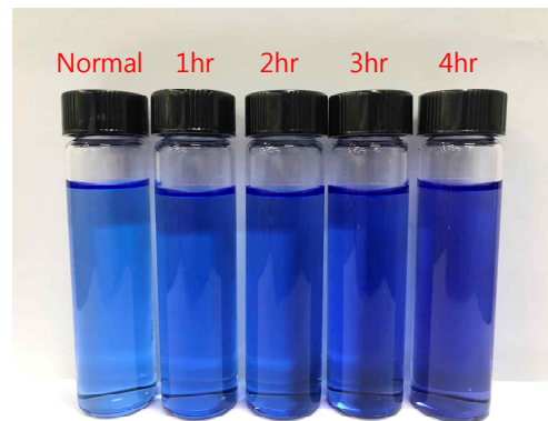
Fig. 3. Samples after biuret analysis according to heating time
