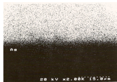
Fig. 5. EDX Ag dot pattern of Ag (upper) / SiC substrate (lower) interface.
