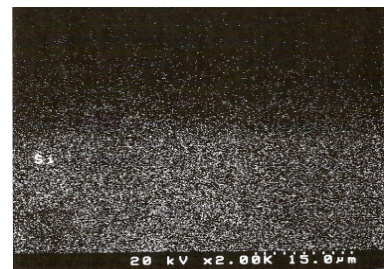
Fig. 6. EDX Si dot pattern of Ag (upper) / SiC substrate (lower) interface.
