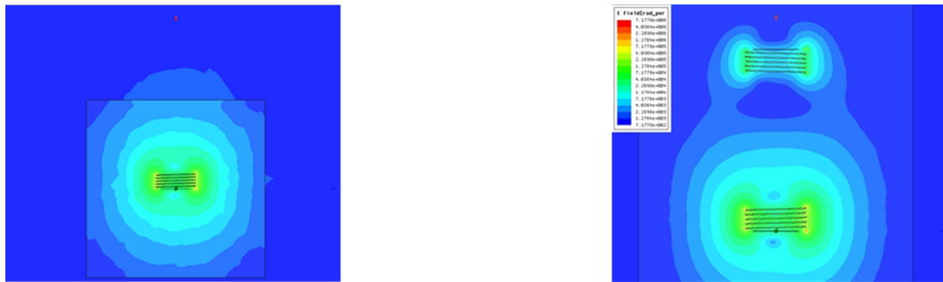
Fig. 7. Distribution of magnetic fields for the magnetic resonant wireless power transfer (WPT)
