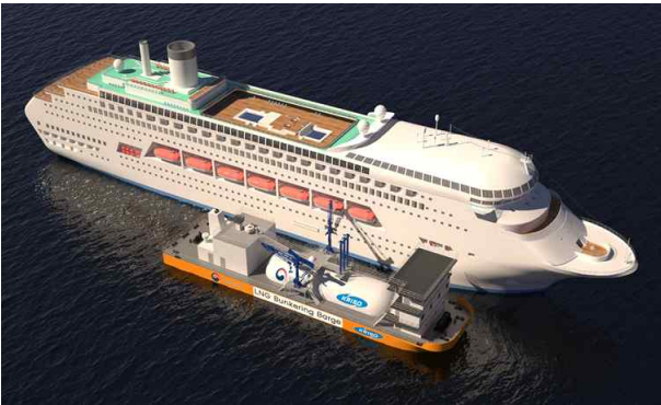
Fig. 1 Ship to ship bunkering using LNG bunkering barge
