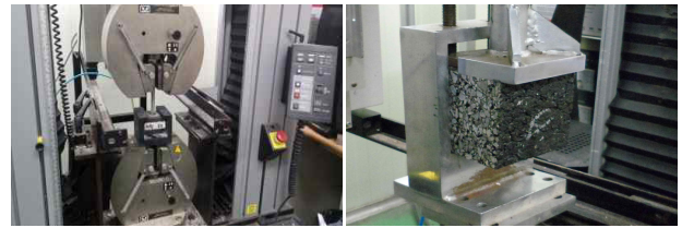
(a) Tensile Adhesion Test (b) Shear Adhesion Test
