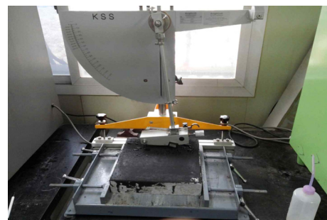
Fig. 4. British Pendulum Tester
