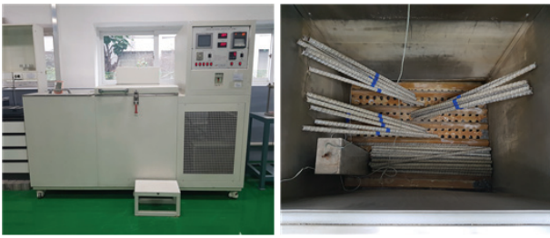
Fig. 2. Equipment of F/T action and the samples inside
