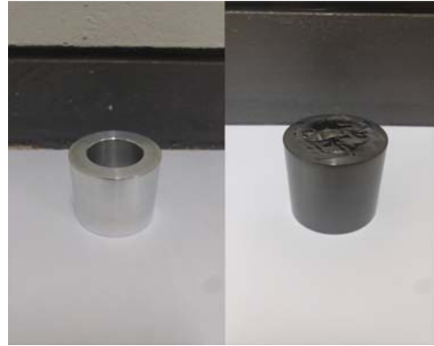
Fig. 1. Polishing & DLC Coating on aluminium cylinder.
