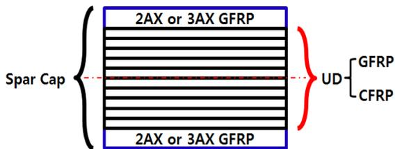
Fig 8 Stacking sequence of spar cap section
