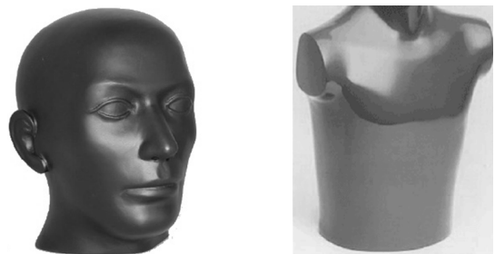
(a) Head & Neck phantom (b)Thorax phantom Fig. 2. Anthropomorphic phantoms of patient and staff (a) Head & Neck phantom, (b) Thorax phantom.
