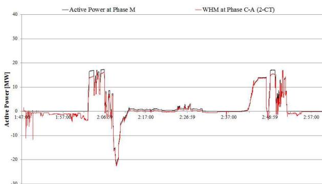
Fig. 15. Watt-hour metering results at phase CA and active power comparison with M phase load
