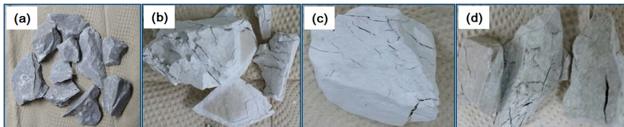
Fig. 1. Natural limestone was calcination at different temperatures (a) Before calcination, (b) Calcination at 900oC, (c) Calcination at 1000oC and (d) Calcination at 1200oC.
