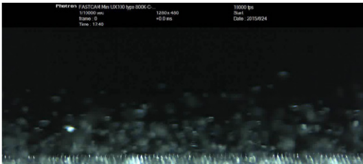
Fig. 9. Distribution of bubbles around surface of micro bubble generator(flow velocity 3 m/s, injection flow rate 30 L/min)
