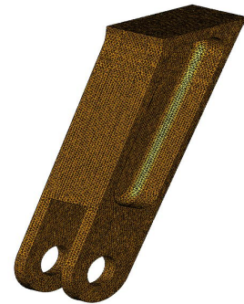
Fig. 5. Finite element model for the hinge beam
