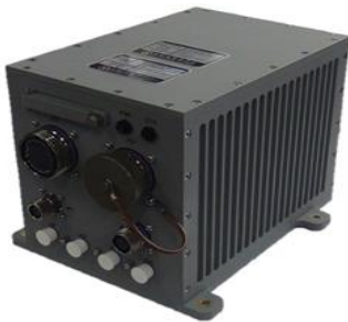
Fig. 2. On-board device of the aircraft load monitoring system [10]
