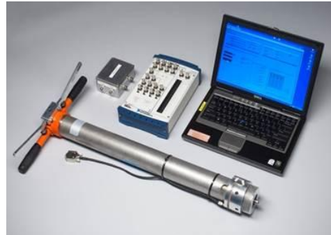
Fig. 4. Mobile impactor for inducing the category 1 damage
