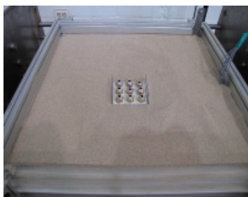
Fig. 6. Group piles installed in the ground
