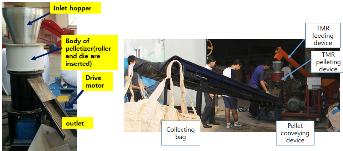
Figure 6. Developed pelletizer and TMR pellet manufacturing system installed in pig farmhouse site
