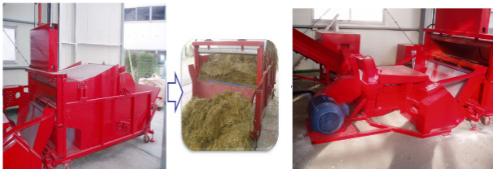
Figure 1. Demolition of round bale and chopping of IRG silage (Hong et al., 2013)
