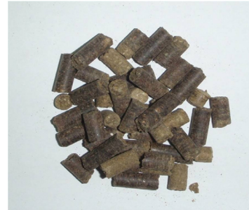
(a) 15-25% moisture content pellets
