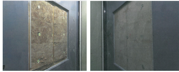
Figure 11. U-factor test of SICIB (for building) (Left: glass wool, right: Inner board (for Building)).
