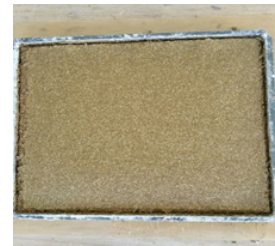
Figure 5. Mixture of pine leaf powder and vermiculite.
