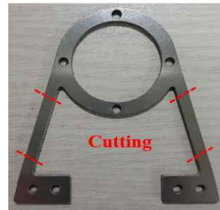
Fig. 16. Sectioning Position for SEM Microscopy
