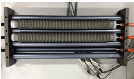
Fig. 3. The measurement of autogenous shrinkage(ASTM C 1698)
