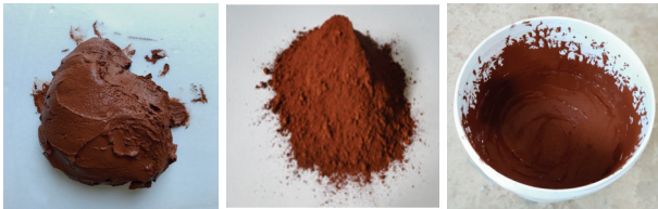
(a) Red Mud sludge (b) Dried Red Mud (c) Liquefied Red Mud
