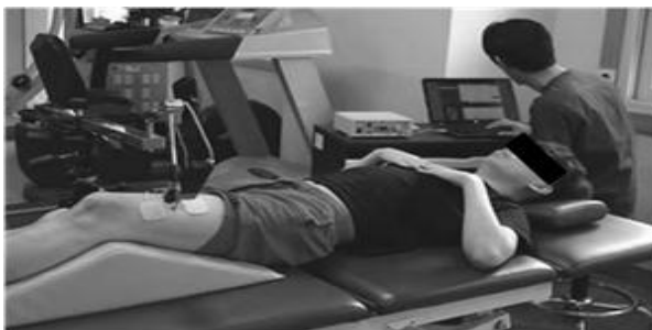
Figure 2. Measurement of the muscle contractile properties on quadriceps muscles using TMG
