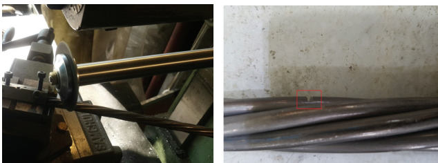
Photo 1 Mechanical damage of 7-wire strand using milling machine
