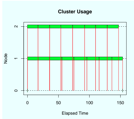
Figure 4.4. Example of the work allocation when applying parallel computing to GCV(h) calculation with two workers ( n = 1000 ). A block represents one allocated workload and a red line represents communication between the master (Node 0) and the worker (Node 1, 2).
