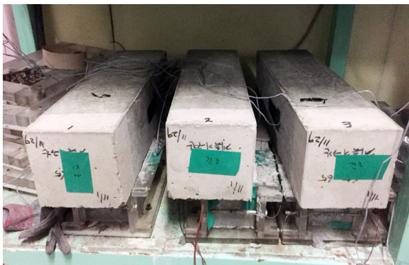
Fig. 6 Laboratory Test for Drying Shrinkage of Concrete
