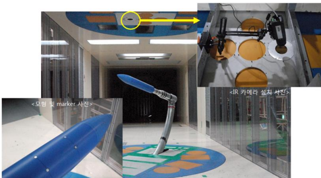
Fig. 1 IR thermography experiment set-up
