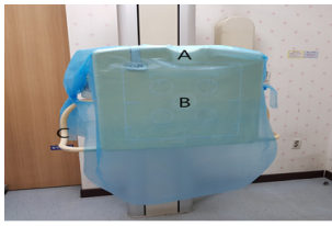
(a) Chin (b) Chest (c) Hand Fig. 3 Area of Chest PA radiography equipment cultured
