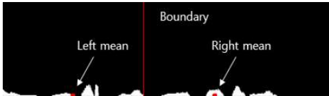
(b) Mean values and boundary obtained by K-means algorithm on the histogram (K=2)
