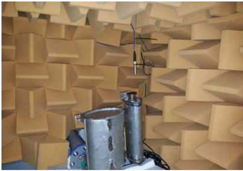
Fig. 4. Noise measurement of 'B' silencer
