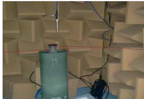
Fig. 3. Noise measurement of 'A' silencer
