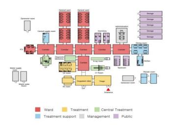
[Figure 12] Posco A&C Level 1 Mobile Hospital Layout
