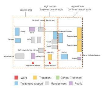
[Figure 10] M.S.F Ebola Treatment Center Plan Diagram
