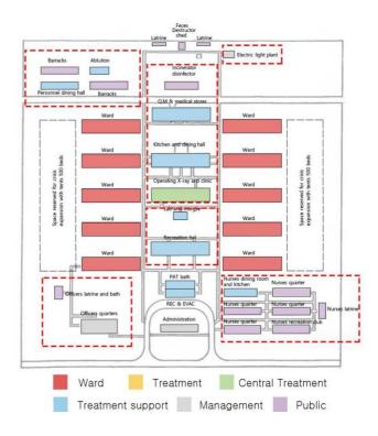
[Figure 1] US Army Field Hospital General layout type A diagram in ww1
