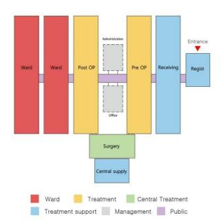
[Figure 5] Basic "U" configuration diagram of MASH(1951) Source: CPT Scott C. Woodard, 2003, The Story of the Mobile Army Surgical Hospital, 509p. (The dotted line worked with estimates.)
