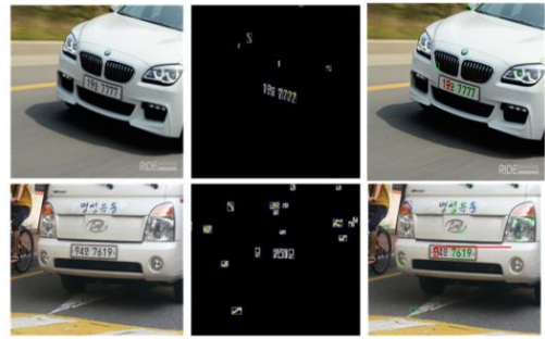
Fig. 13. Vehicle images where there are different characters from images with slanted plates (a) Original image (b) Outline extraction image (c) License plate area estimation result image
