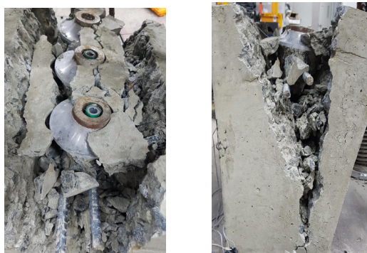
<Fig. 7> Crack and failure of test specimens
