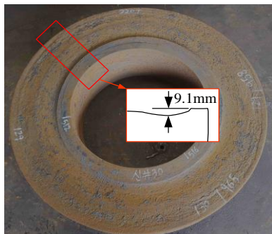
Fig. 7 Groove of L-shaped ring rolling in process line
