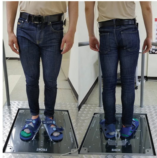
Fig. 1. The experimental posture for measuring the LOS and the static postural balance on balance training system with LLD.
