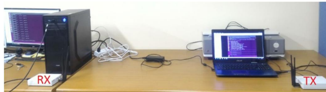
Figure 3. PU transmitter and SU receiver with USRP hardware and GNU Radio software
