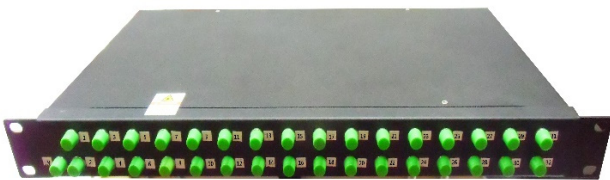
FIG. 5. The photo of the fabricated 32-port cascaded encoder enclosed in 1U chassis with FC/APC connectors. 1 input port and 32 output ports can directly connect the DF link with FC/APC.
