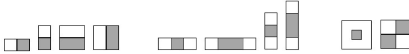
Figure 2.2. Haar features; (left) Edge feature, (middle) Line feature, (right) Center surrounded feature and special diagonal line feature.
