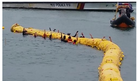
Fig. 6. Buoyancy test for adults holding onto lifelines attached to both sides of oil boom.
