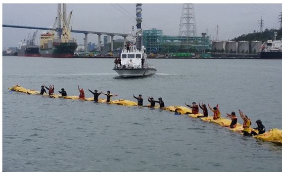
Fig. 8. Buoyancy test by the group of three adults riding on the top of oil boom.
