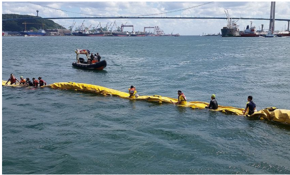
Fig. 7. Buoyancy test for adults riding on the top of the oil boom.
