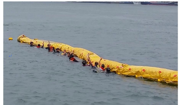
Fig. 5. Buoyancy test for adults holding onto lifelines attached to one side of oil boom.
