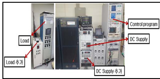
Fig. 7. The equipment of anti-islanding evaluation for power conditioning system connected in parallel.
