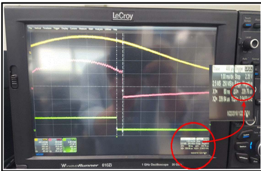
Fig. 12. The picture of oscilloscope that evaluated power conditioning system when grid-off.
