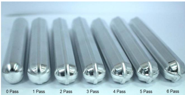
Fig. 2 Images of workpieces depending on forging passes
